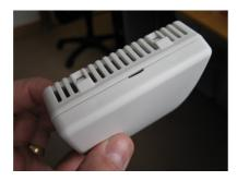
Figure 2. .By pressing a flat screw-driver into the opening slot, the two locking hook would be released.
