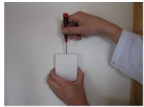
Figure 2. .Hold the top cover and slowly separate the top and base housing.
